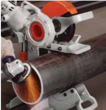
Model 258 with Pipe Roller in use for beveling. Two operators are recommended for this operation
